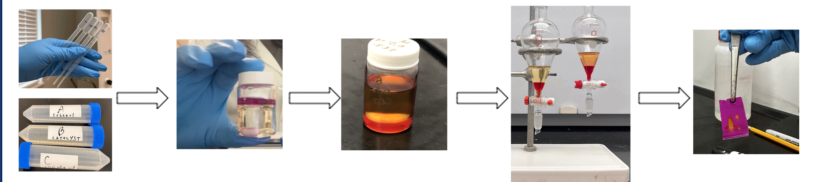
Figure 4: The process of making biodiesel at the classroom scale (10g), showing phase separation and TLC quality control.
