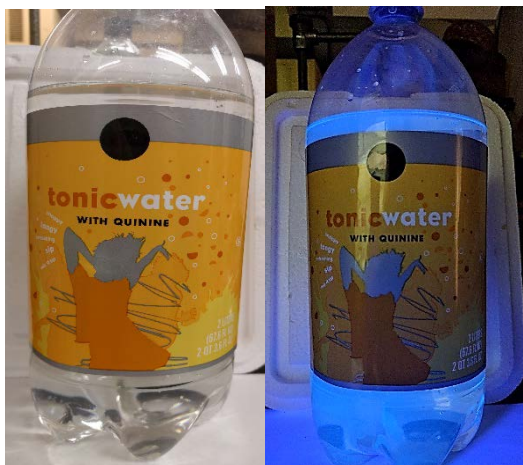
Figure 1: At left, tonic water seen under normal classroom light. At right, the tonic water when illuminated by the black light.
