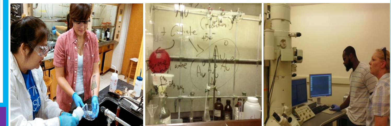
Teacher and graduate student rinsing slides after working with piranha bath solution. Reaction mechanism for gold nanoparticle growth sketched by graduate student. Graduate student setting up the transmission electron microscope while a teacher observes.
