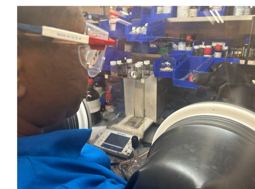
\text{Co}_4\text{S}_4(\text{PR}_3)_4 Synthesis inside nitrogen glovebox.
