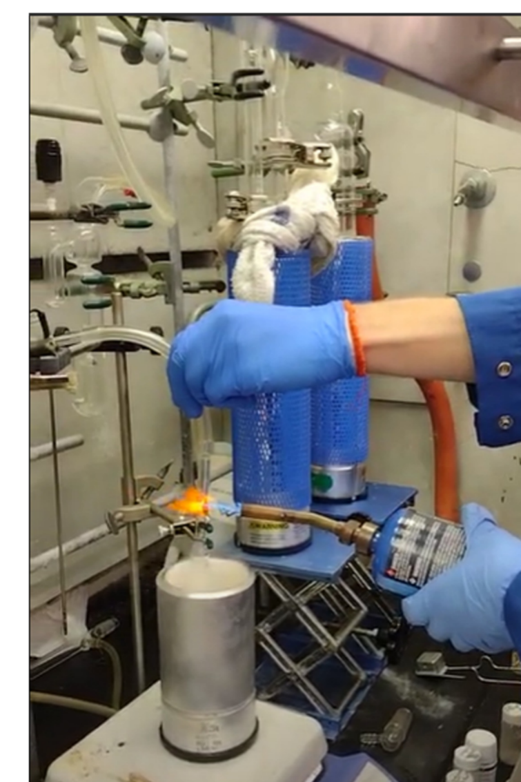
Vacuum Sealed tube for COF synthesis
