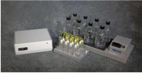
Figure 6—EBS Challenge respirometer system for wastewater treatment monitoring http://www.ebsbiowizard.com/2012/05/respirometry-as-a-tool-for-troubleshooting-of-biological-wastewater/
