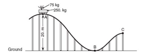
Compare the total mechanical energy of the car and passenger at points A, B, and C.
