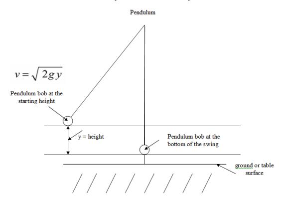
At the post lab discussion, we will compare the predicted speed and actual speed of the pendulum bob. The class data will verify the assumption of conservation of energy that we made at the beginning of the lesson when we equate the potential energy at the top and kinetic energy at the bottom. The next day, the students will do guided and individual practice problems on conservation of energy. The worksheets on conservation of energy are found in the appendix.
