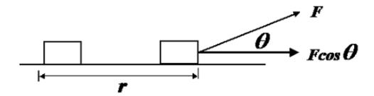
Here the F' and cos' part of the equation is the component of the applied force that is in the direction of the displacement.
