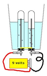
This picture shows a possible apparatus for electrolysis of water<sup>11</sup>. However, in the experiment description above, the test tubes are suspended into the beaker with the use of j-shaped copper wire which wraps around the edge of the beaker and then into the test tubes.
